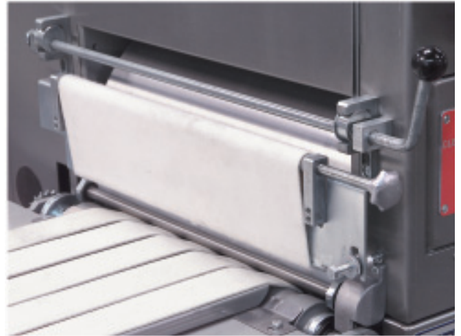
Adjustable turning flap for transfer with seam up
