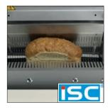
Intelligent Slicing Concept (JAC patent) Continuous automatic control system that slices loaves according to their consistency. This allows open textured,
