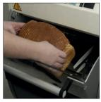
Front safety cover Locked during the slicing process for maximum safety.
